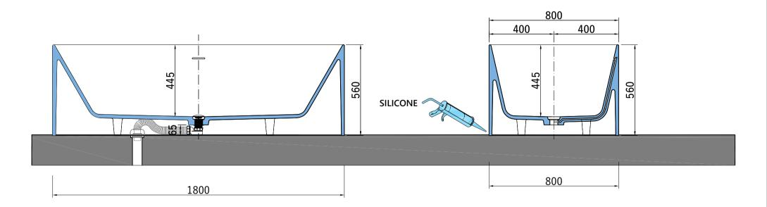
**N.B.** For correct installation, we recommend using polyurethane foam between the bathtub and the floor.
